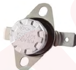
RAC4586 TERMOSTATO BAQUELITE KSD301 250V 10A 75° NF
